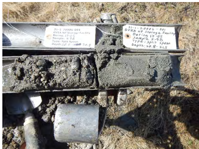
Photograph 28: Sample S-9a and S-9b, boring 17-05, 20.0 feet bgs to 21.5 feet bgs.
