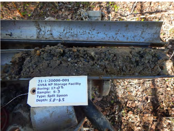
Photograph 9: Sample 3, boring 17-02, 7.5 feet bgs to 9.0 feet bgs.
